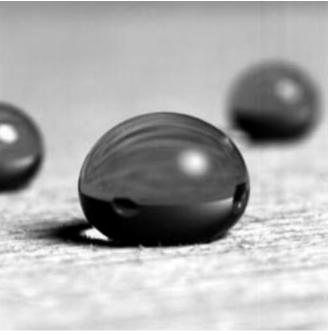
Source: BASF - Wood surface repels water droplets. 2002 Fig. 4.- Drop formation on a hydrophobic surface.
