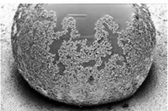
Source: BASF - The lotus effect keeps the leaf surface clean. 2002 Fig. 5.- Drop of water whith dirt particles on a hydrophobic coating.
